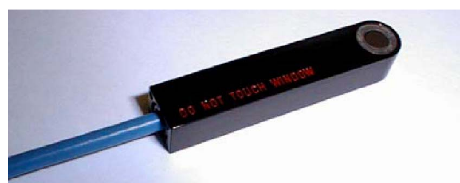
Fig. 2a PTW model T34013 ionization chamber with dimensions on schematic drawing.
